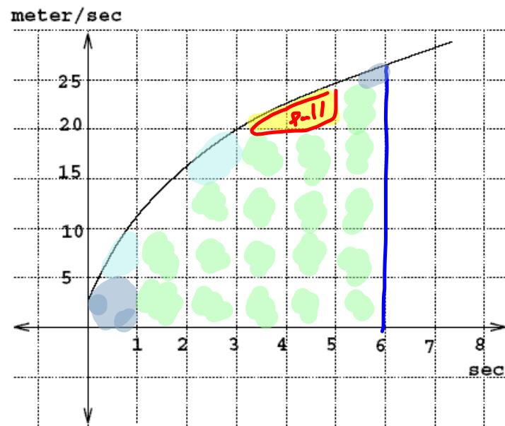
Each box on the grid has an area of  $(1)(5)=5$  or distance of 5 meters
